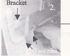
D. 3. In the back (pull the tube over the rib)
